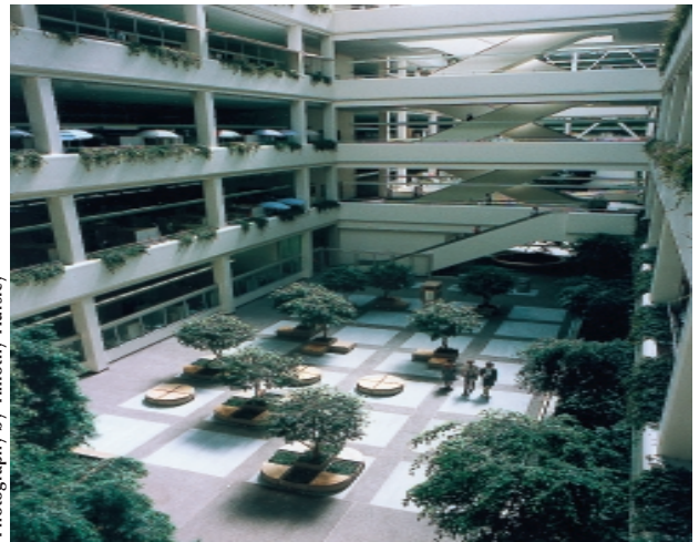
The “litetrium” in the center of the building creates an open, expansive feeling. Daylight from overhead provides ambient lighting for the surrounding office areas.
