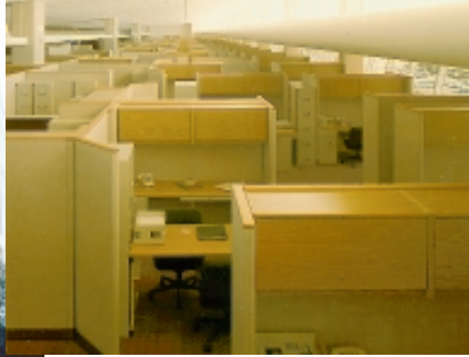
Daylight entering the building reflects off the internal light shelves and the sloped ceiling to provide diffuse ambient lighting deep into the work areas.
